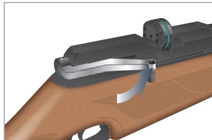
4. Close and lock the bolt by pushing the bolt handle forward. **Do not load more than 1 pellet into the barrel. Immediate shooting after cocking is recommended to prevent loading of 2 pellets into the barrel.**
