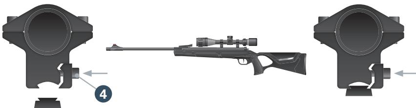
4. Loosen the fixing screw **4** of each mount and set the riflescope (with the mounts fitted as described) onto the dovetail rail of the gun, then secure the assembly in place with the fixing screws.
